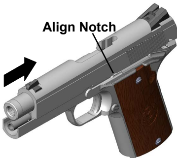
Figure 2a: Slide Catch Notch Alignment
