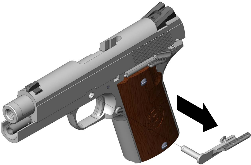
Figure 3: Slide Catch Removal
