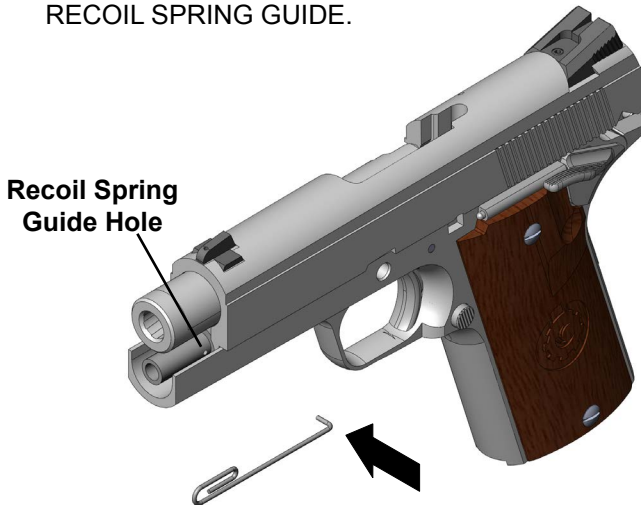
Figure 4: Insert Take Down Tool (or Paperclip)
