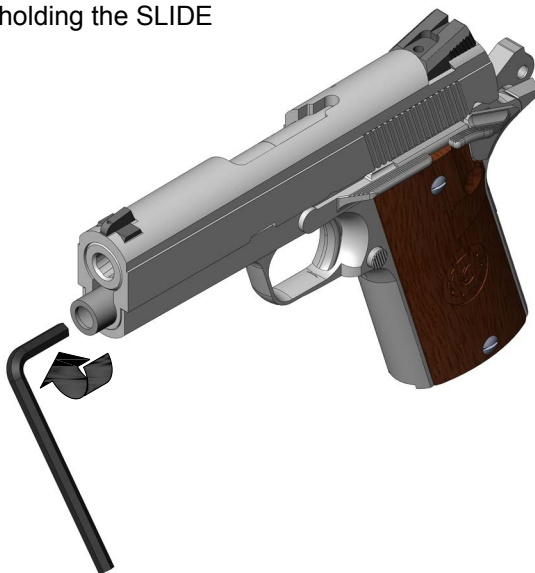
Figure 9: Rotating Recoil Spring Guide
