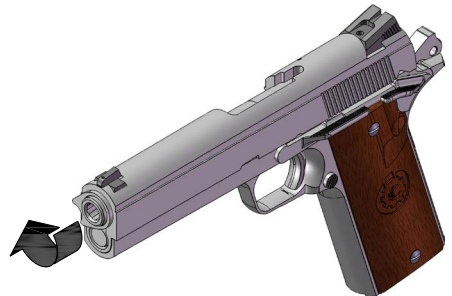
Figure 3: Barrel Bushing Clockwise Rotation
