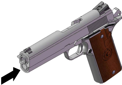
Figure 2: Recoil Plug Depression
