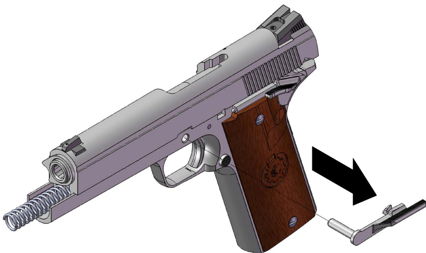
Figure 6: Slide Catch Removal
